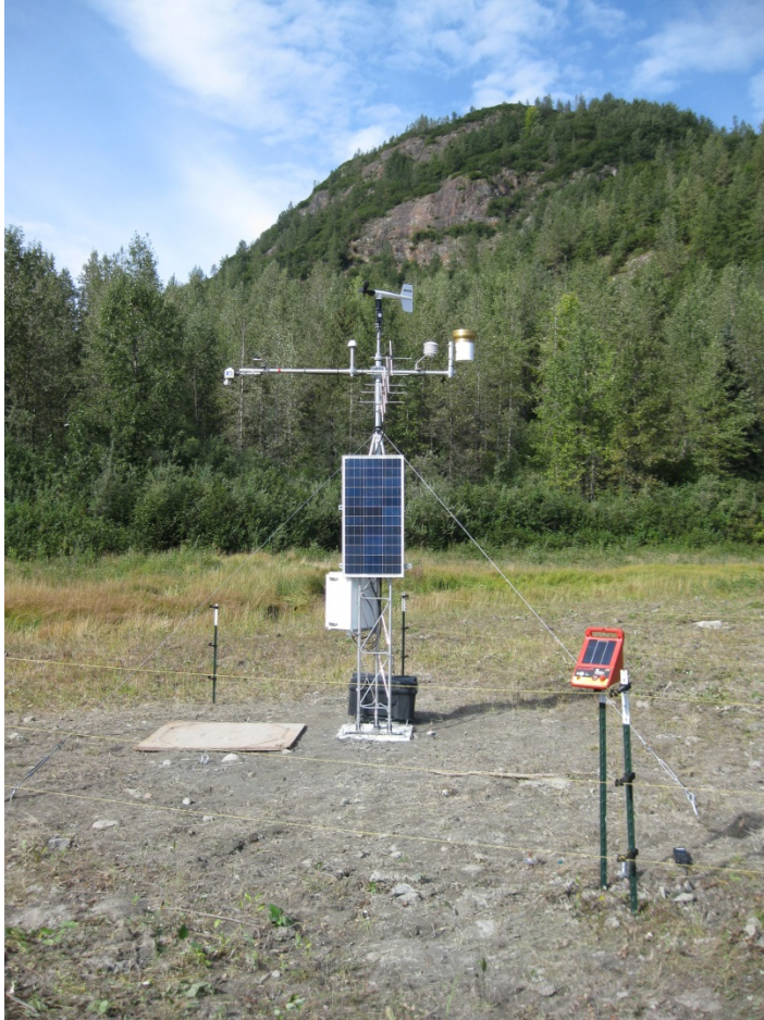
Figure SOP 8-2. Network weather station (tower configuration) with electric fence.
