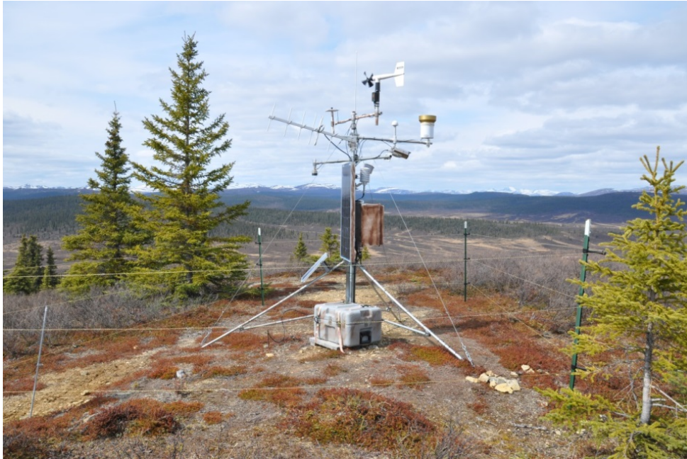
Figure SOP 8-1. Network weather station (tripod configuration) with electric fence.
