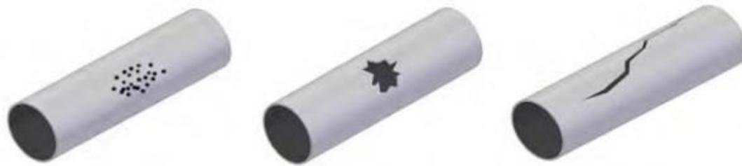
Exhibit 2. Three common types of pipe damage (Reliable Pipes & Tubes LTD. 2018).
