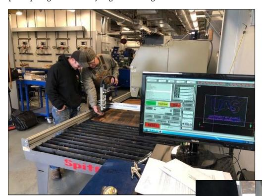
The Welding Program just installed a computerized plasma cutter for the lab. The CNC plasma cutter uses the computer guided wand to precisely cut out any image you want. Pictured above are Ken Horn and Ryan Houtcooper practicing with the machine. To the right is a close up of the cutter's accuracy.
