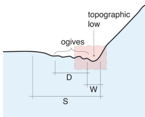
**Fig. 8.** An idealized schematic of lake ogives and the topographic basin in which they form. Three geometric definitions are given to describe the morphology.  $S$  refers to width of the full extent of the lake basin (i.e. the larger topographic basin),  $W$  refers to the width of the ephemeral lake, and  $D$  refers to the downstream length of the ogive train. The highlighted red box is the section of the geometry that is the focus for the conceptual model in Figure 9.
