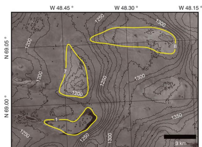
**Fig. 5.** Digital elevation model (DEM) produced from SPOT5 imagery acquired on 2 August 2008, with 10 m contours in black. Lakes 1, 7 and 8 are outlined, and SPOT5 visual imagery is also shown. These lakes are located in the same geographic positions in aerial photos taken in 1985 (Motyka and others, 2010).
