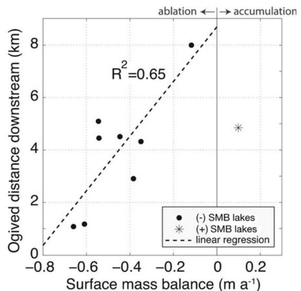
**Fig. 10.** A selection of eight lakes observable in the SPOT5 visual imagery. The ogived distance downstream,  $D$ , is measured from this imagery and plotted against the surface mass-balance (SMB) values,  $\dot{b}$ , interpolated from the Ettema and others (2009) dataset. A linear regression is performed only for the lakes with a net annual ablation (negative SMB).
