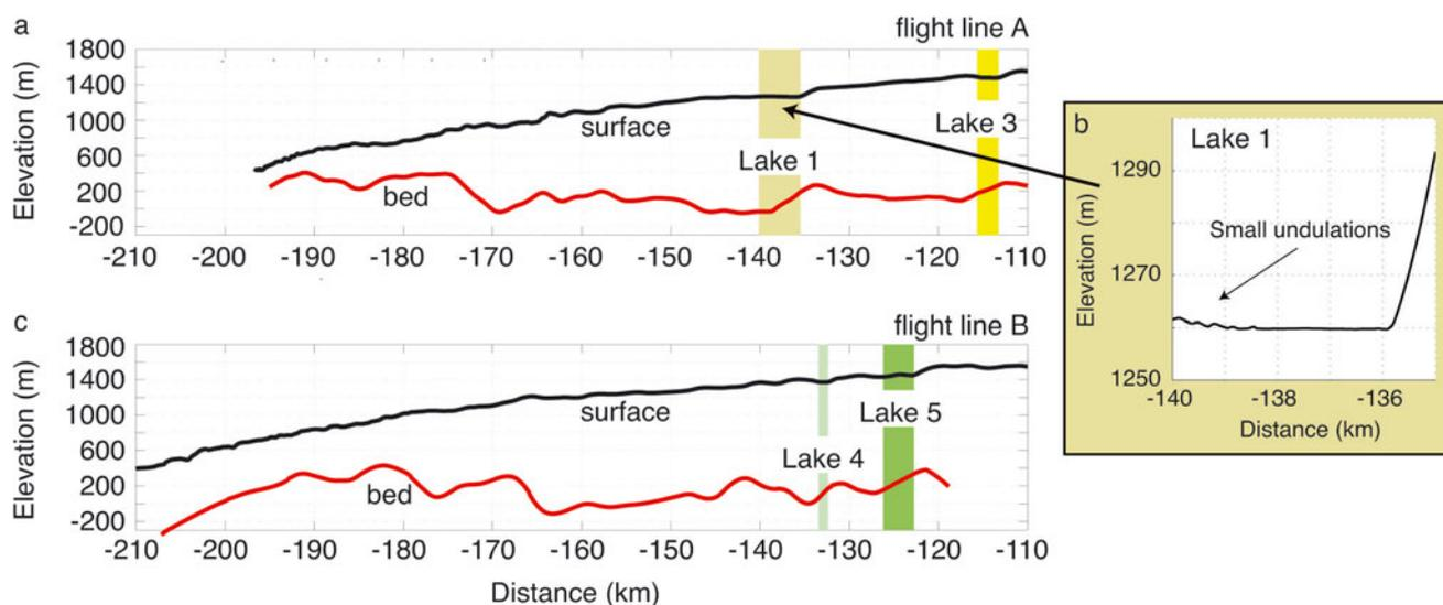
**Fig. 4.** (a, c) Flight lines A and B, respectively, indicated in Figure 2b. Surface (black line) and basal (red line) topography on along-flow transects that cross lakes with ogives. (b) Darkened panel shows enlarged surface topography at Lake 1. Surface topography is from NASA ATM data. Bedrock topography from the CReSIS multichannel coherent-radar depth sounder was smoothed with 1 km averaging window.
