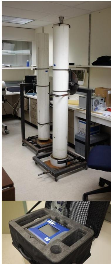
Figure 2-1. The dustfall column and the aerosol sensor used to record data for the UAFDUST application.
