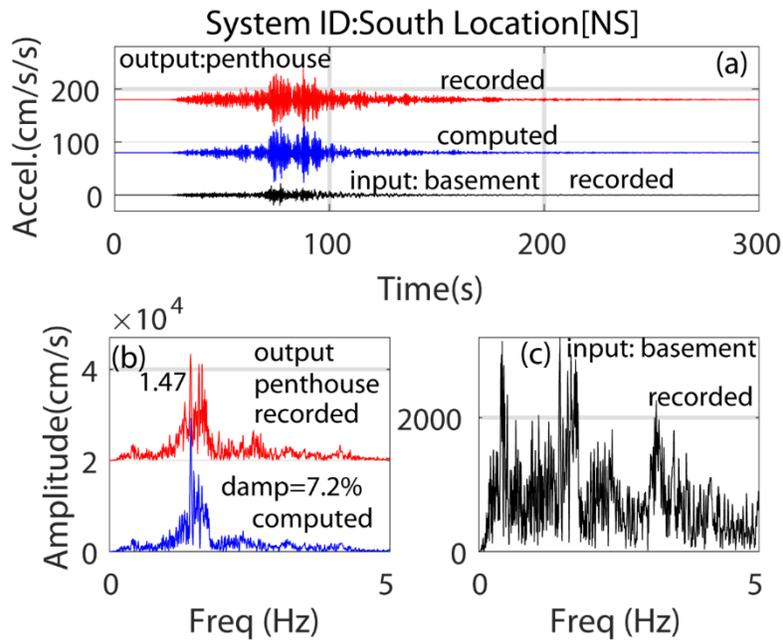
**Figure 8.** System identification of NS accelerations at south locations. (a) NS channels at the south basement location and penthouse are used as input and output, respectively. The plot also shows the computed penthouse acceleration using the ARX method. (b) Amplitude spectra of recorded and computed accelerations at the penthouse. (c) Amplitude spectrum of acceleration at the basement used as input.
