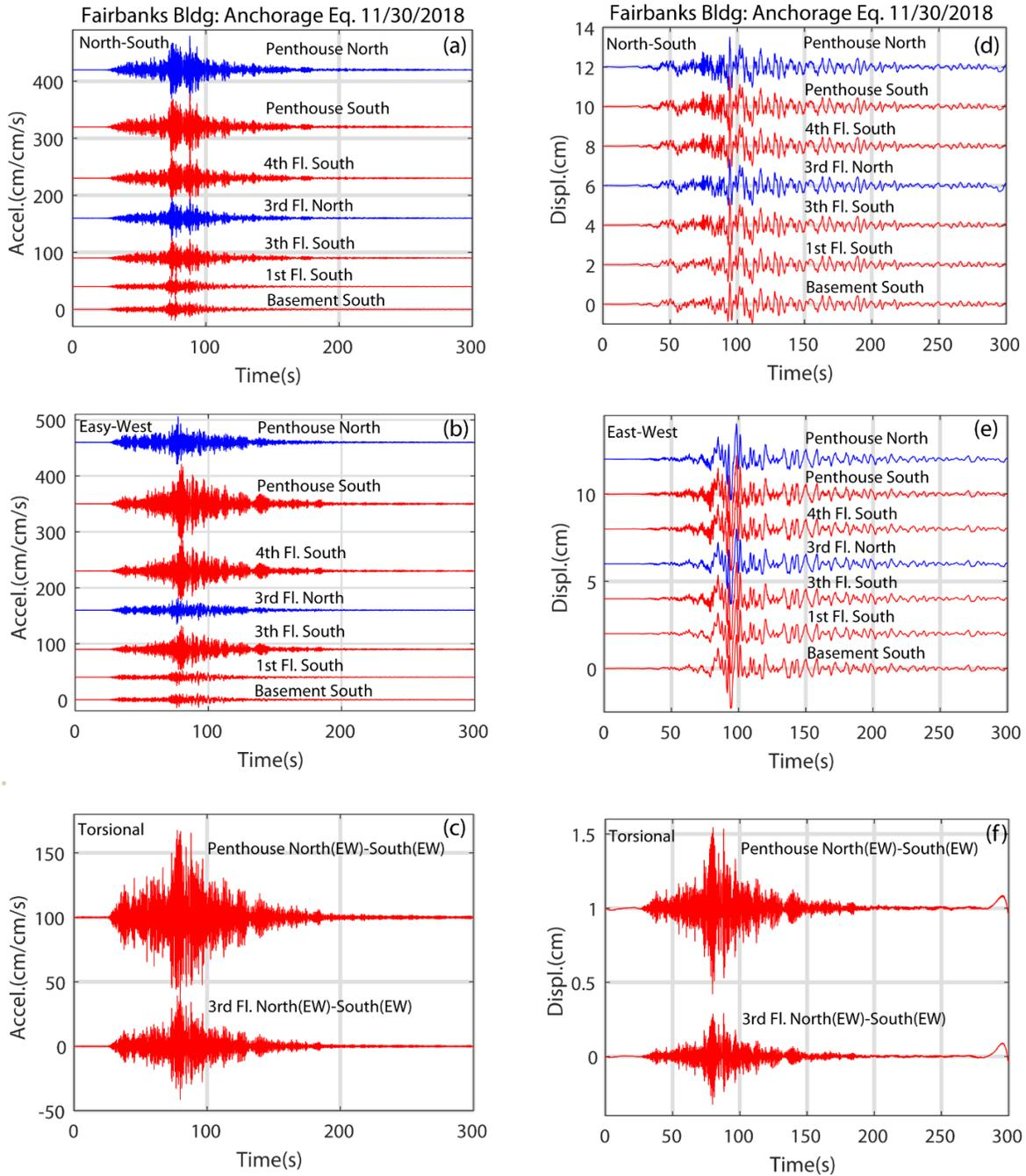
**Figure 4.** Panels a, b, and c show NS, EW, and torsional acceleration time-histories, respectively. Panels d, e, and f show NS, EW, and torsional displacement time-histories, respectively. Time histories in red are from channels in the south location and those in blue are from channels in the north location.
