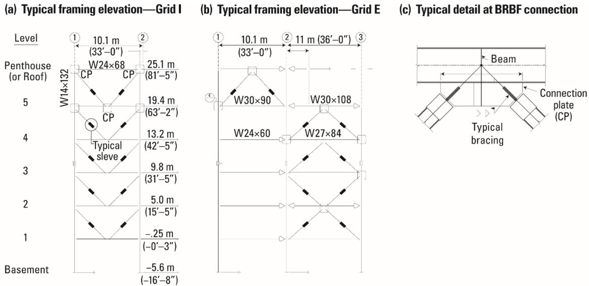
**Figure 3.** (a and b) Typical buckling restrained braced framing (BRBF) elevations depicting K-bracing with BRBs and typical details at (c) connections and connection plates (CPs). (Figure developed using information in structural blueprints of the building).
