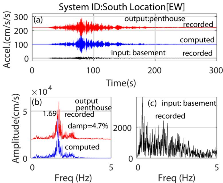
**Figure 9.** System identification of EW accelerations at south locations. (a) EW channels at the south basement location and penthouse are used as input and output, respectively. The plot also shows the computed penthouse acceleration using the ARX method. (b) Amplitude spectra of recorded and computed accelerations at the penthouse. (c) Amplitude spectrum of acceleration at the basement used as input.
