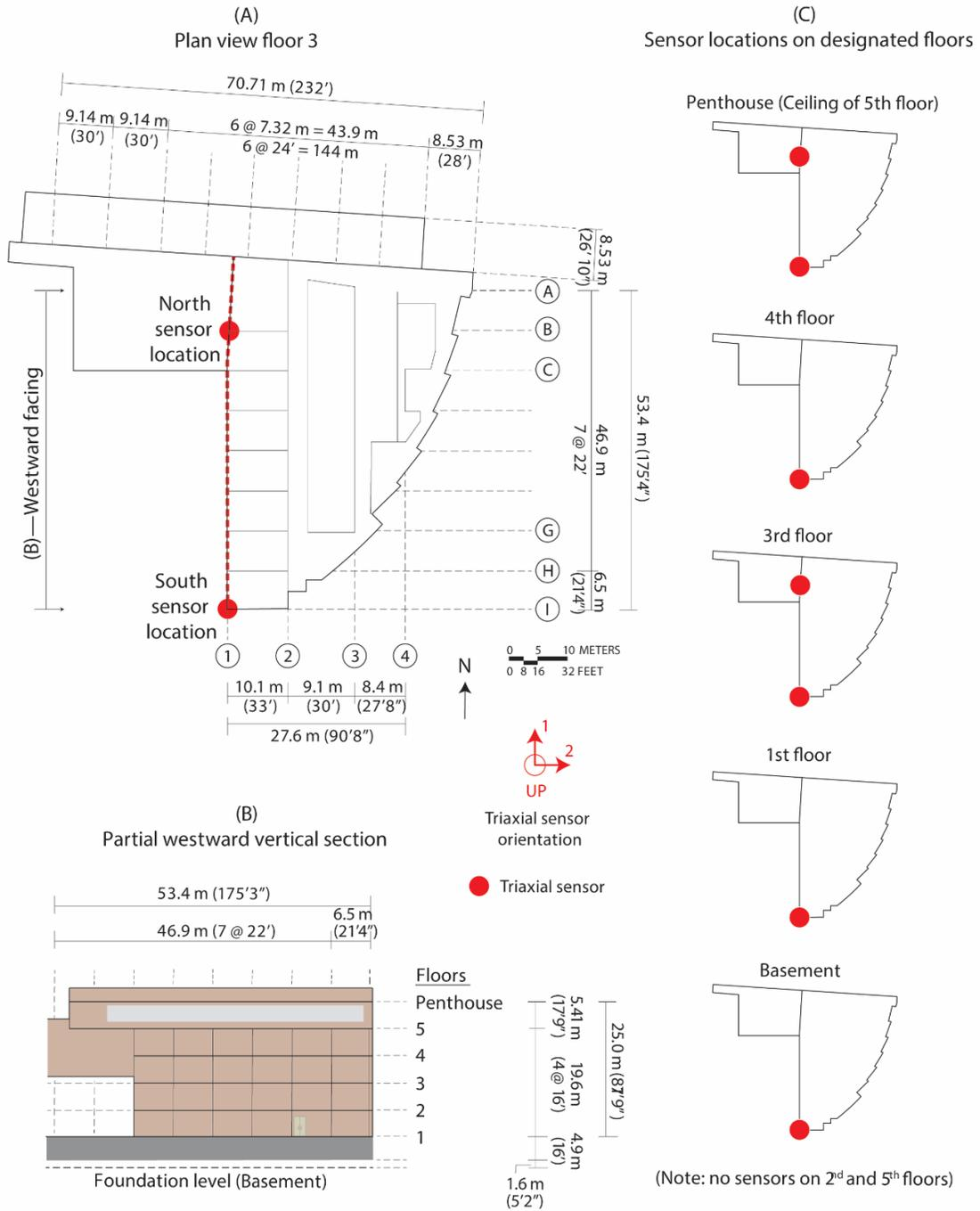
**Figure 2.** General schematic plan views, a vertical section of the building, and monitoring array. (A) Plan view of the building (3<sup>rd</sup> floor) indicates that channels oriented as 1 (NS) are all on grid line 1 and those oriented as 2 (EW) are all in either Grid Line I or B or both as described in (C). (Figure developed using information in structural blueprints of the building).
