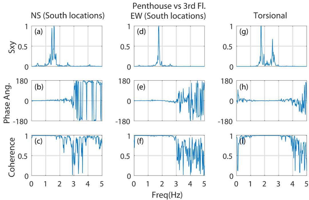
**Figure 6.** (a, d, g) Cross-spectra, (b, e, h) phase angles, and (c, f, i) coherency plots for (a, b, c) NS, (d, e, f) EW, and (g, h, i) torsional accelerations recorded at the penthouse and 3<sup>rd</sup> floor.
