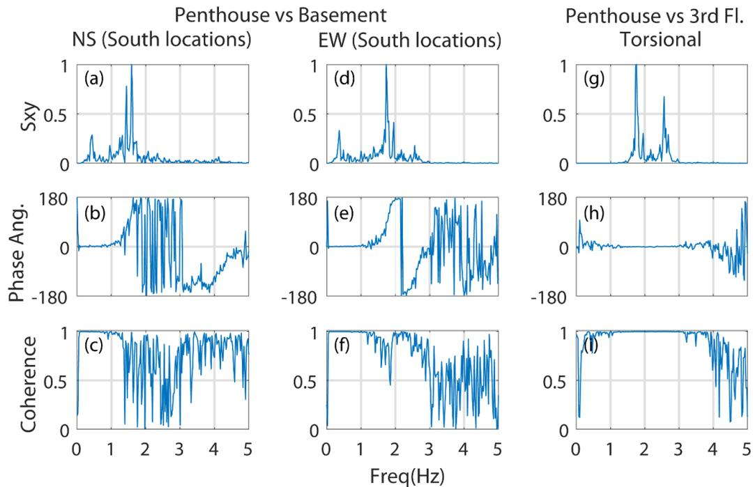
**Figure 7.** (a, d, g) Cross-spectra, (b, e, h) phase angles, and (c, f, i) coherency plots for (a, b, c) NS, (d, e, f) EW, and (g, h, i) torsional accelerations (recorded at the penthouse and basement for NS and EW and penthouse and 3<sup>rd</sup> floor for torsional).
