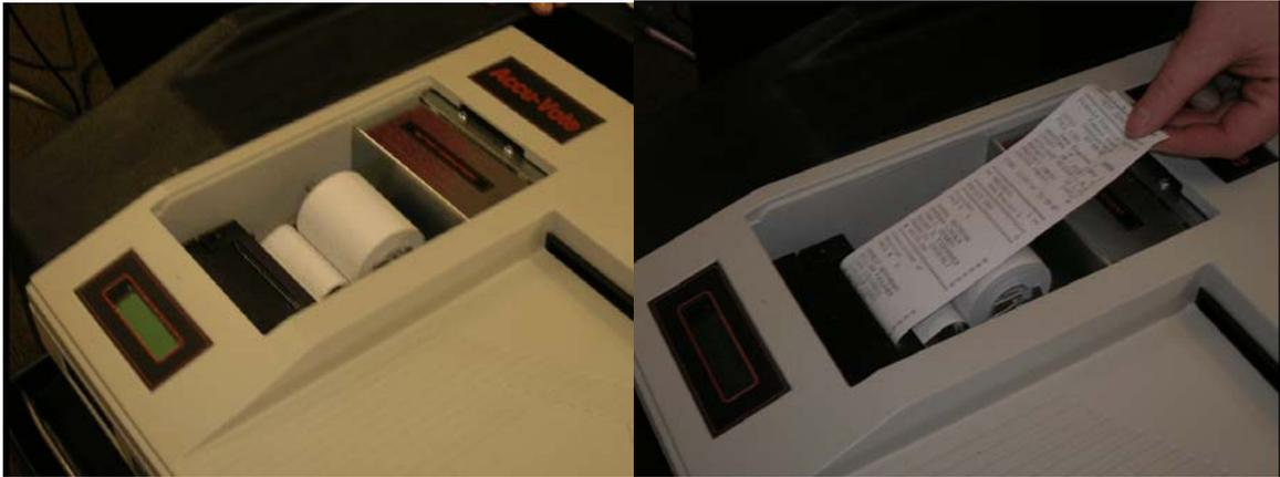
AccuVote-OS Terminal positioned over ballot container. Note lockable panel on ballot box is opened (lower left) . During election, locked front and rear panels of the ballot box cover the secured memory card port and the rear of AccuVote-OS unit (lower right).
