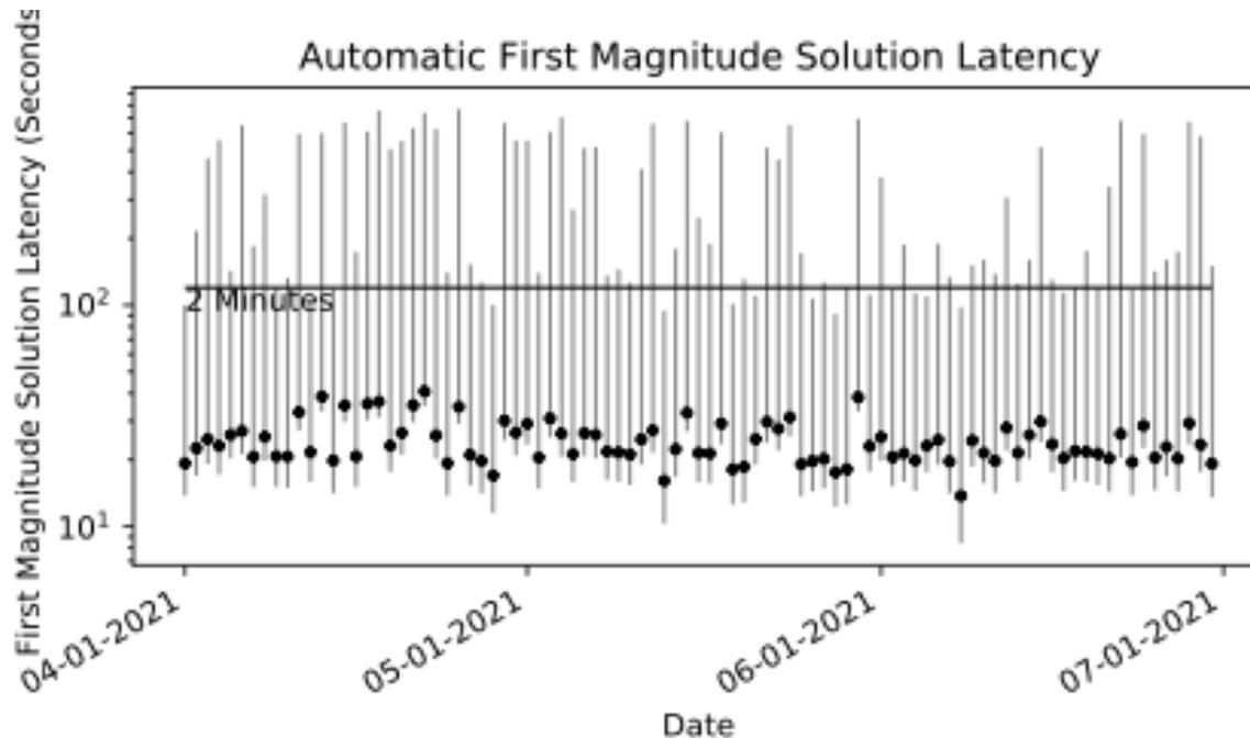
**Figure 5.3.** Average daily latency (dots) and range (lines) of first automatic magnitude for each event after the event detection.
