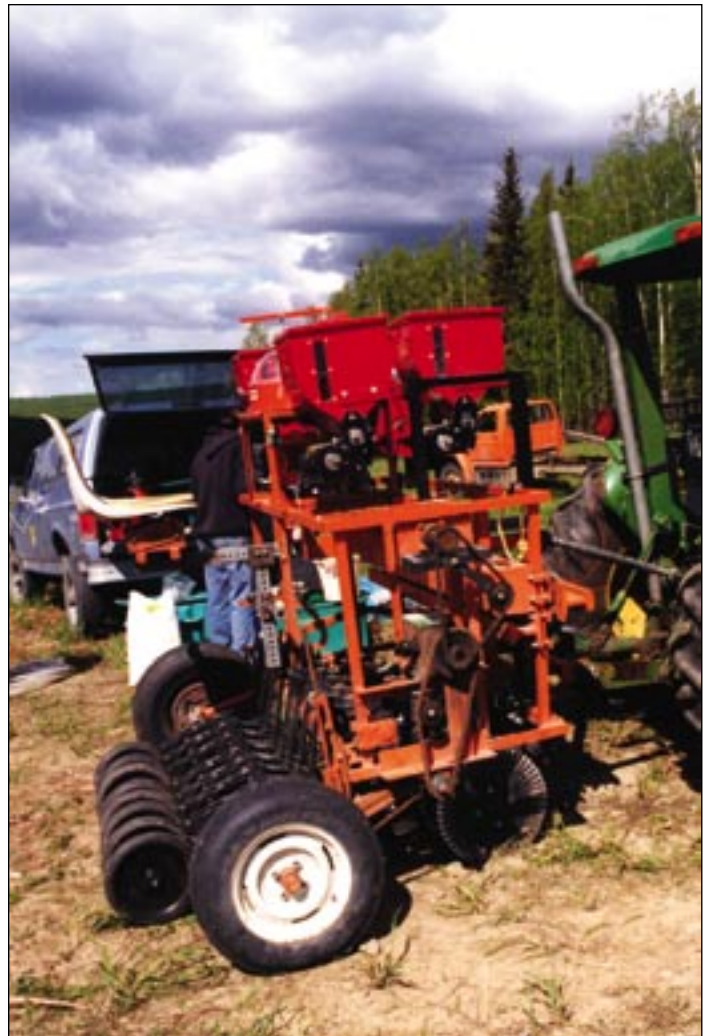
Plot drill, built by Dan Hall at the Matanuska Experiment Farm, used to compare seeding forage crop into untilled and tilled soil.
