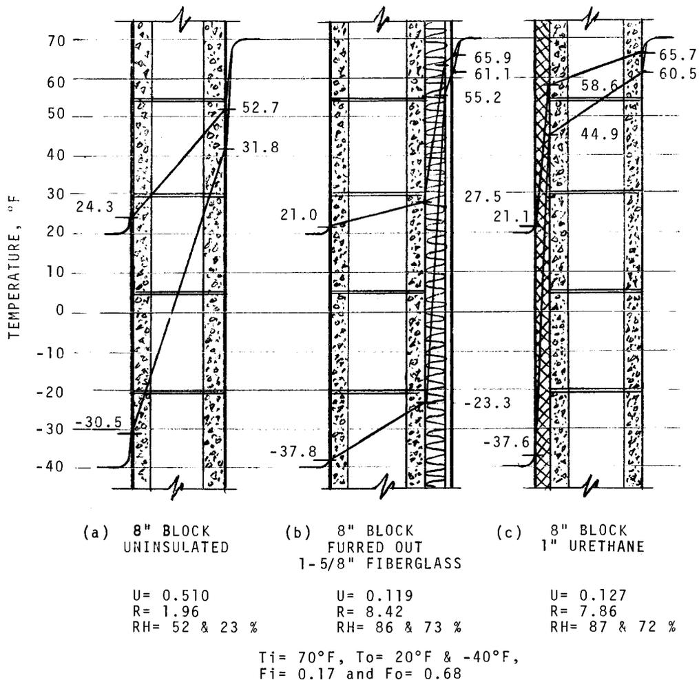
FIGURE 1. TEMPERATURE GRADIENTS OF MASONRY WALLS
