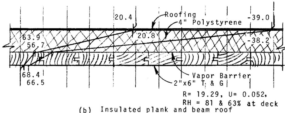
(b) Insulated plank and beam roof
