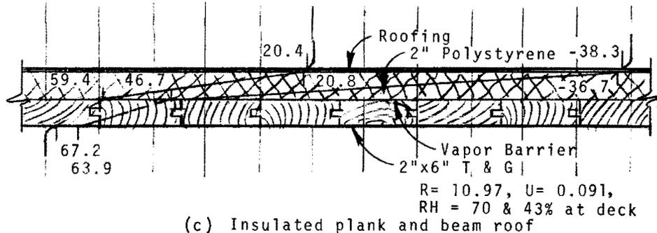
(c) Insulated plank and beam roof
