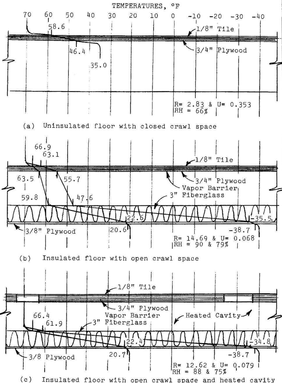
FIGURE 3. TEMPERATURE GRADIENTS OF FLOORS
