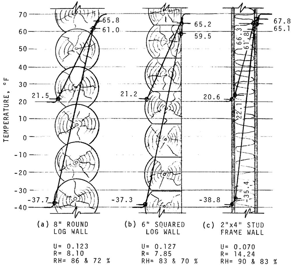
FIGURE 2. TEMPERATURE GRADIENTS OF WOOD WALLS
