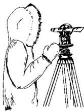
theodolite cannot sight on Polaris in northern Alaska without special eyepiece prisms or other equipment. Also, during much of the year the sun is so low that refraction uncertainties are very serious, and the relationships of horizontal to vertical angles are very poor. Standard PZS triangle methods on any star will work, but this doesn't help the surveyor who has been trained to work solely with azimuth shots on Polaris at elongation.
