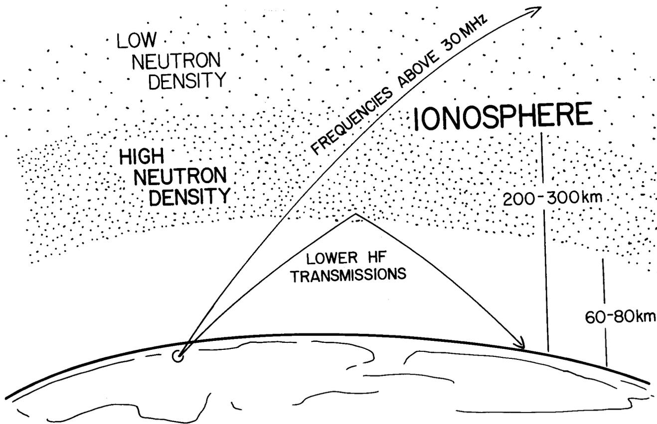
**High frequency radio signals propagate through the ionosphere with ease, while low frequency radio signals are absorbed and reflected in the ionospheric region.**
