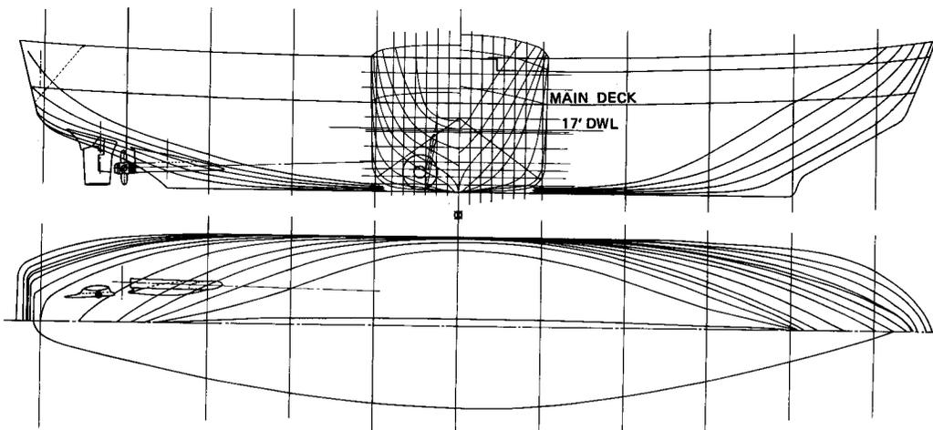
Hull lines of ice-strengthened polar research vessel.
