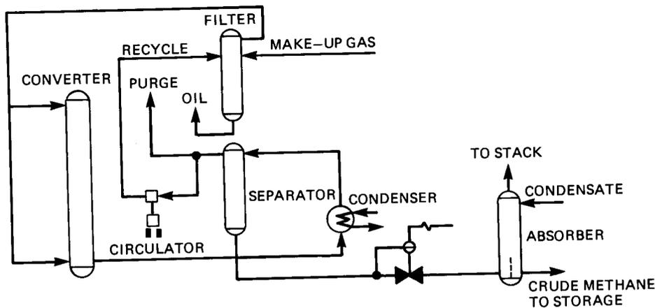
Figure 3. Schematic flow diagram for medium-pressure methanol synthesis.
