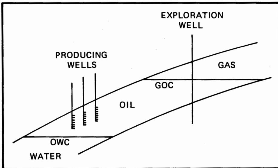
Figure 1. Reservoir configuration showing gas, oil and water zones and contacts. Note successful completions in the oil zone.
