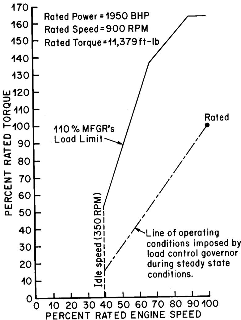
Left: Torque-speed characteristics of proposed diesel engine (900 rpm rating).
