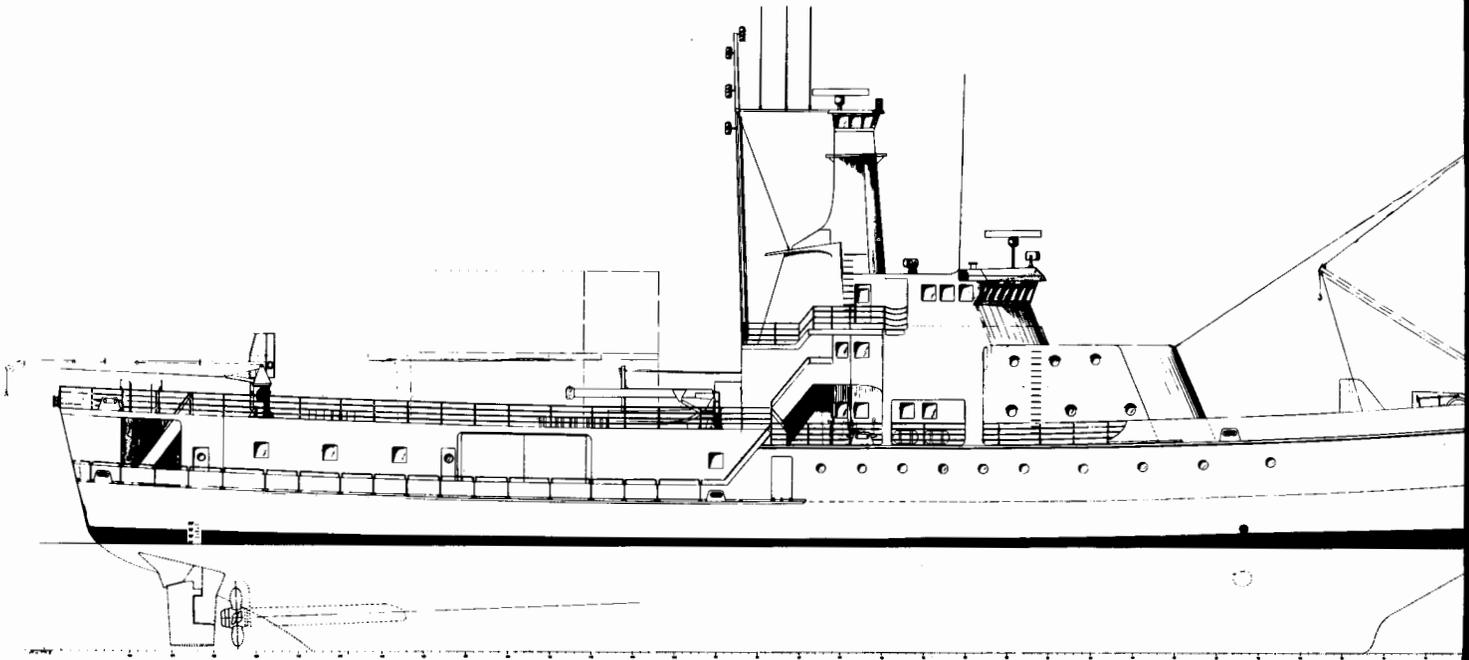
Outboard profile of ice-strengthened polar research vessel. (Illustrations courtesy of the authors.)
