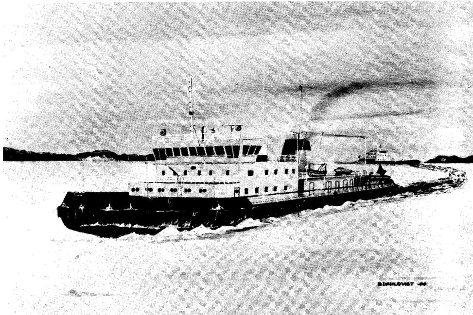
The vessels will be equipped with diesel-electric machinery, with the primary power being supplied by three diesel engines each developing 1605 kW (2180 horsepower). These engines drive AC generators supplying four 950 kW (1292 hp) DC propelling motors over thyristor rectifiers. Main particulars are: length max. 76.8 m; breadth max. 16.6 m; draught 2.5 m; and shaft output 3800 kW (5170 hp).
