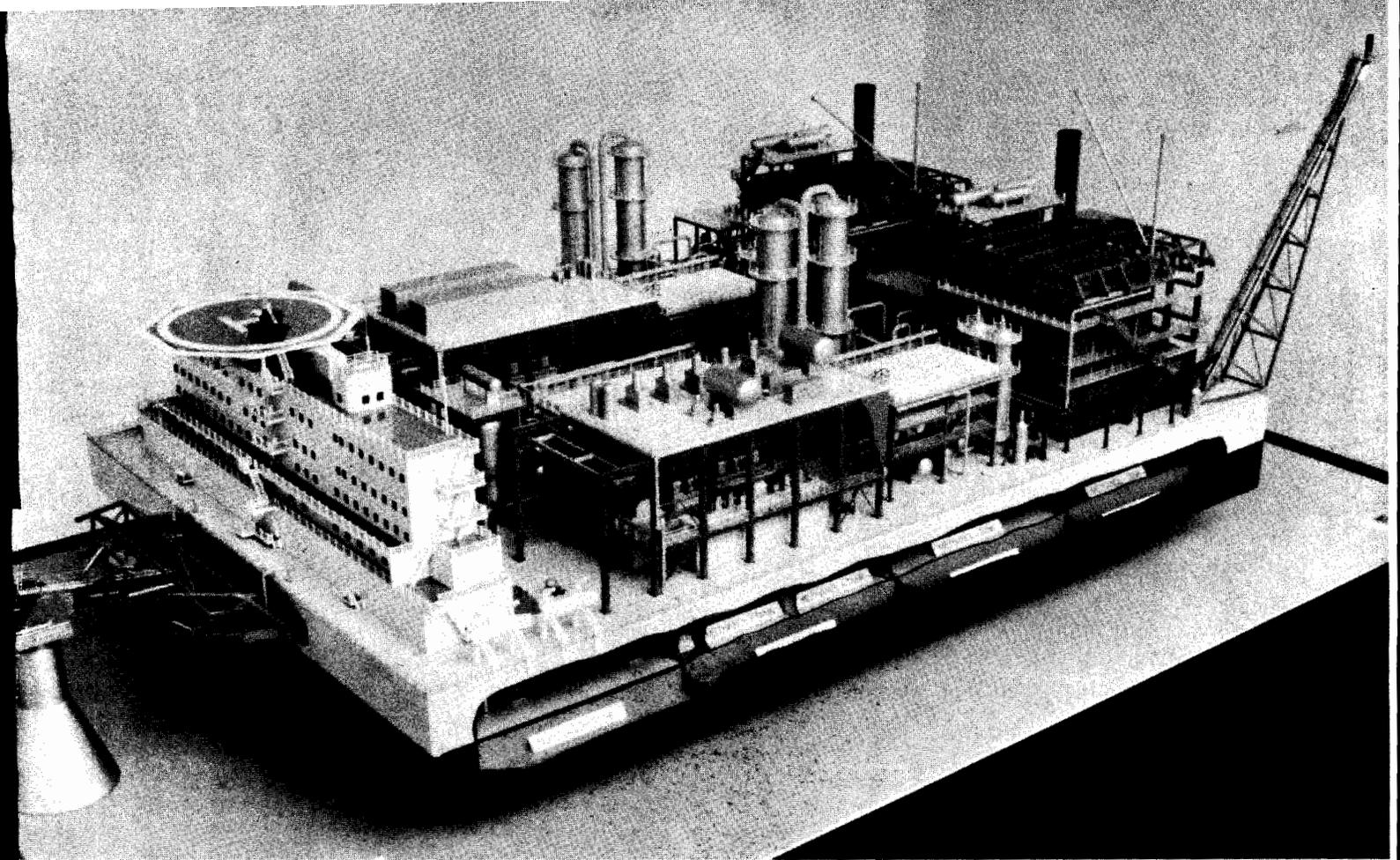
Figure 2. Model of barge-mounted methanol production train. (Photo courtesy of Litton Industries.)
