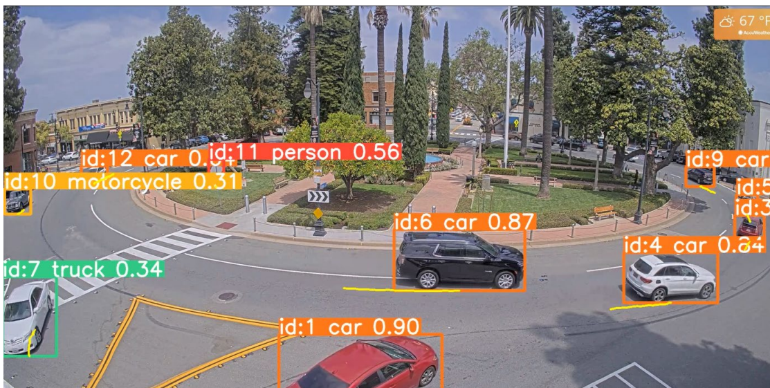
Figure 2.2 Example misclassified car as truck and motorcycle.
