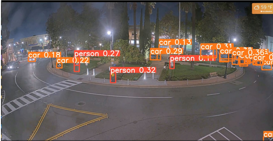
Figure 2.3 Example of misclassification of inanimate objects during low lighting.
