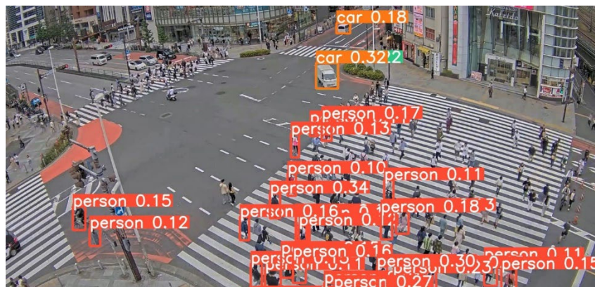
Figure 3.6 Example of a high level of pedestrian detection.
