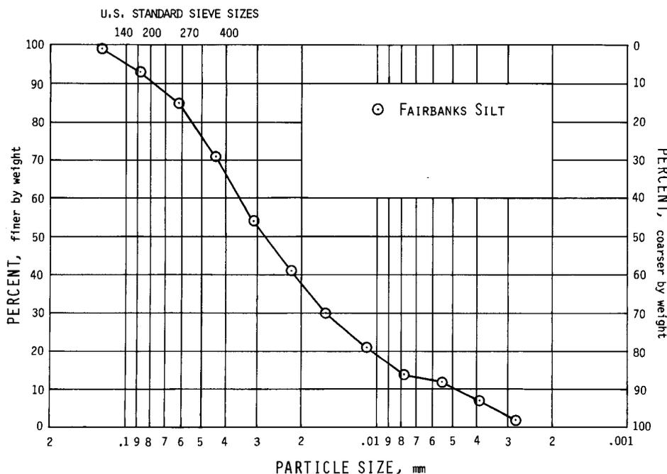
Figure 4. Particle-size distribution for Fairbanks silt test soil.
