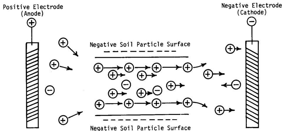
Figure 3. Illustration of electro-osmotic flow in an electric field.
