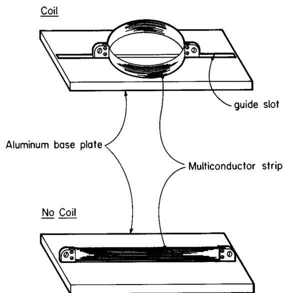
Figure 1. Snap-ring magnetometer design, showing the flexible multiconductor strip and sliding handles. The coil can be changed from a finite cross-sectional area (top view) to zero by sliding the handles outwards.
