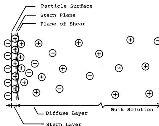
Figure 1. Ion distribution at and near the soil particle surface.<sup>5</sup>
