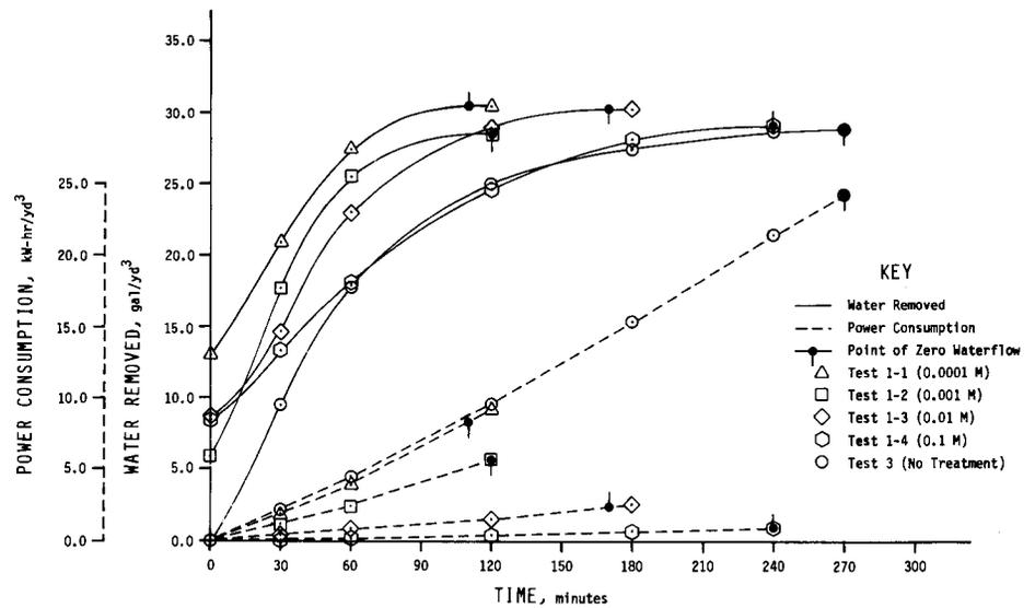
Figure 6. Dewatering and power consumption curves for laboratory tests using ferric chloride ( $\text{FeCl}_3$ ) in soil treatment. Amounts of decant prior to electro-osmotic dewatering procedures are represented at time zero.
