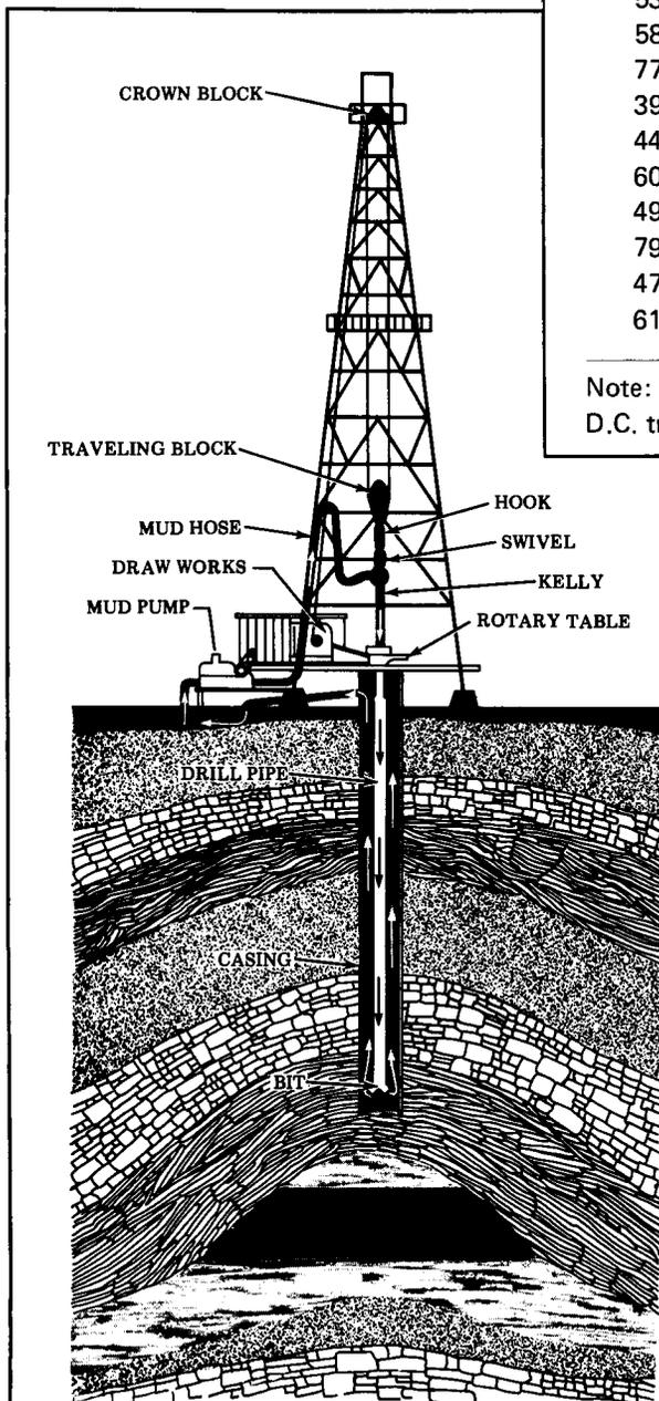
Schematic illustration of a rotary drilling rig showing the flow of drilling fluid used to clear drilled material from the bottom of the hole and to maintain pressure for the purpose of avoiding gushers or blowouts. (From Energy/Alaska by Neil Davis, UA Press, in press.)
