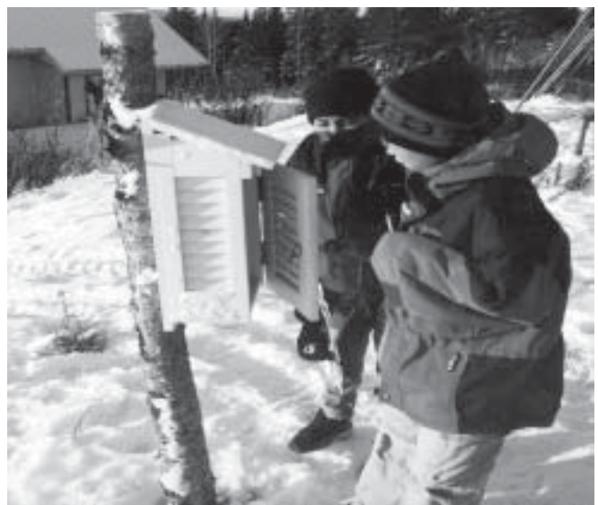
Students take current, minimum and maximum daily temperature readings within one hour of solar noon.
