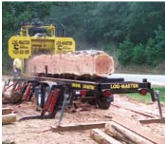
Portable sawmills, like this Log-Master 5, may help reduce labor costs. See story on page 22. —PHOTO COURTESY LOG-MASTER PORTABLE SAWMILLING MFG., INC.
