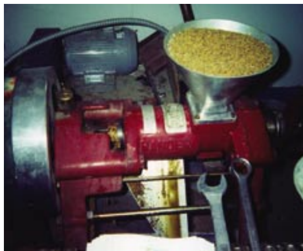
Canola press used to extract oil, located at the Agricultural and Forestry Experiment Station, Fairbanks Experiment Farm.
