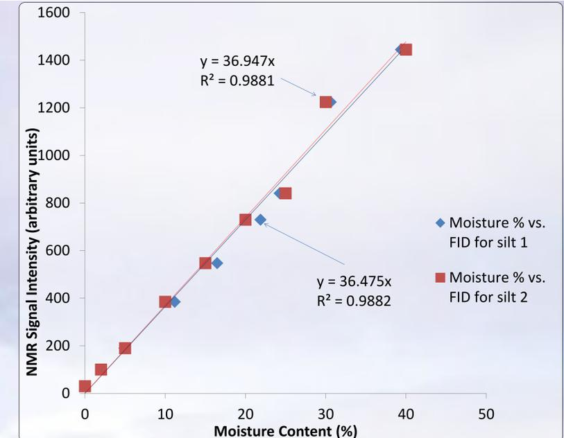
Figure 4. NMR signal intensity for duplicate silt samples with corresponding moisture content.
