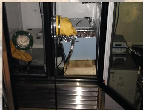
Figure 1. Temperature control system (NMR on the left and cooler on the right in the refrigerator, respectively, and temperature bath on the right outside of the refrigerator).
