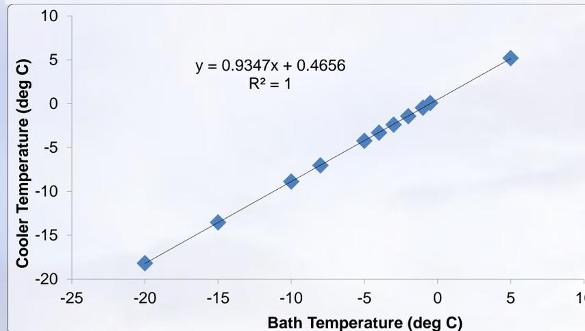
Figure 2. The linear relationship between cooling bath temperature and cooler temperature.
