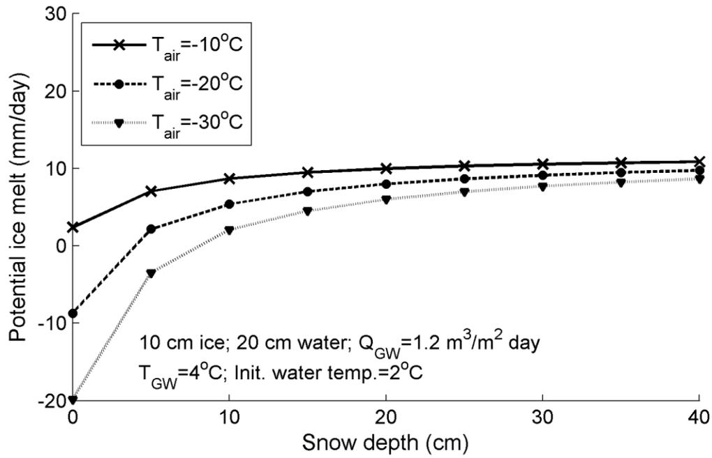
Figure 3.10. Potential ice melt with varying snow depths at different air temperatures.
