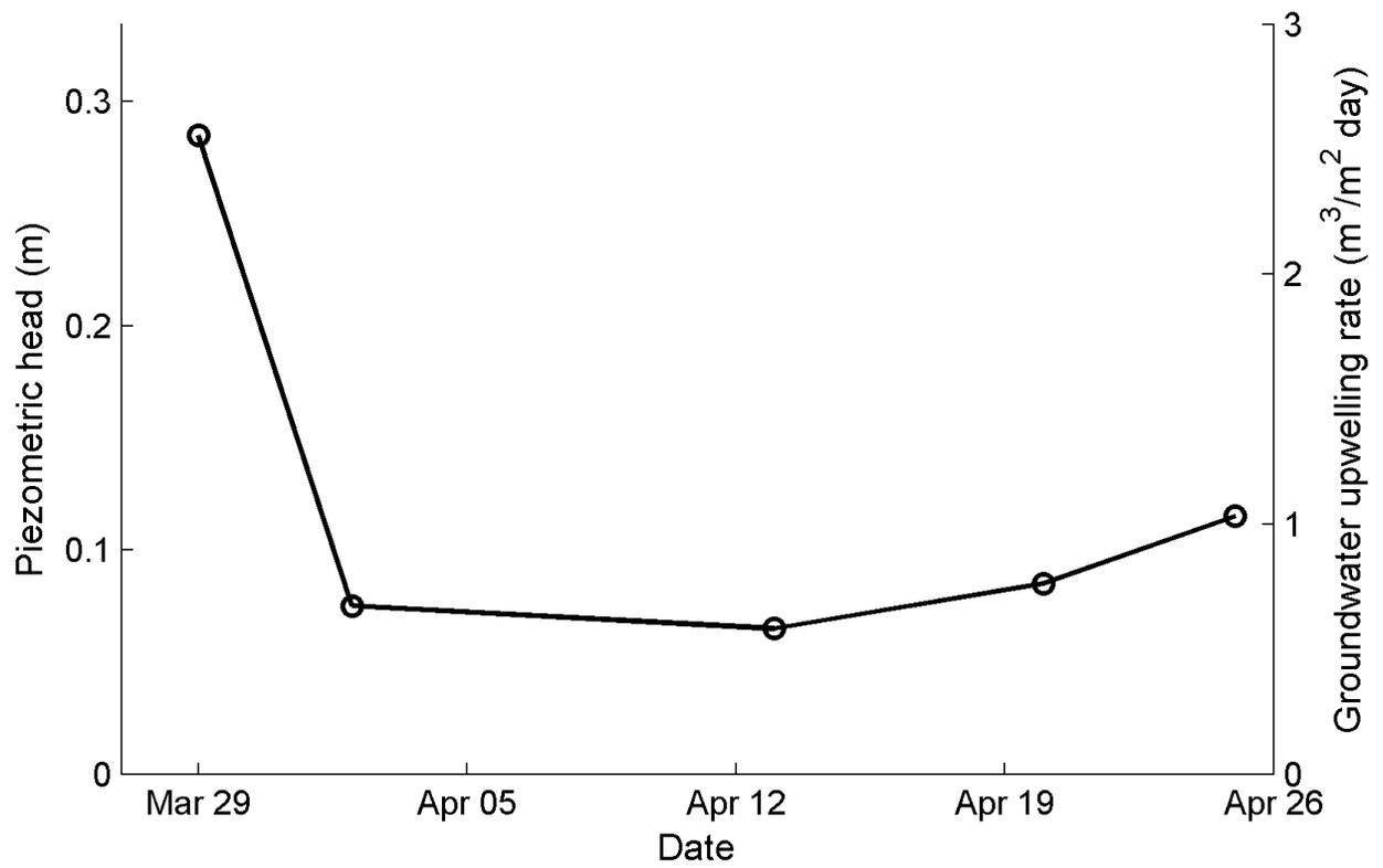
Figure 3.4. Piezometric head and groundwater upwelling rate as measured 1.10 m beneath the channel bottom of Hot Cake Slough of the Tanana River.
