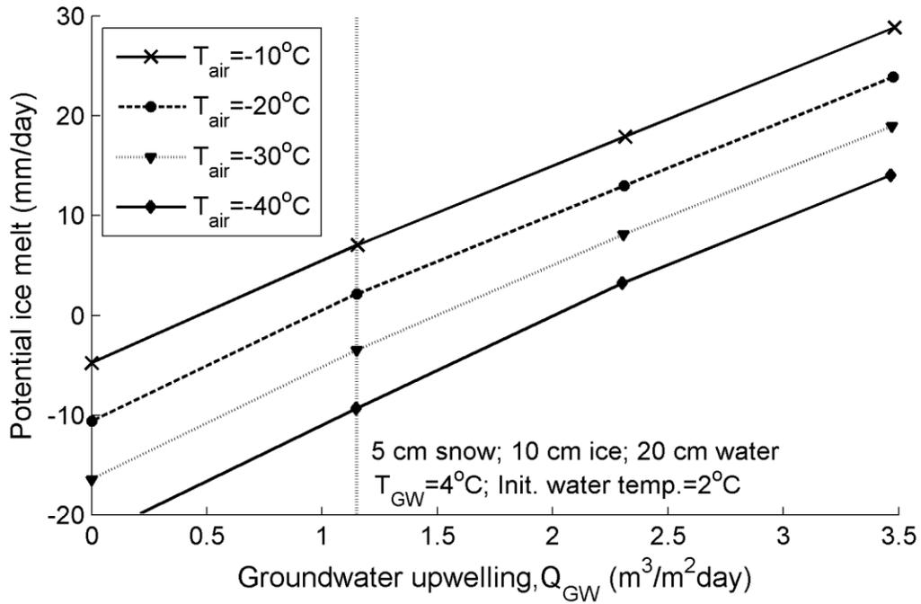
Figure 3.8. Potential ice melt with varying upwelling rates at different air temperatures (or rate of thickening when ice melt rates are negative).
