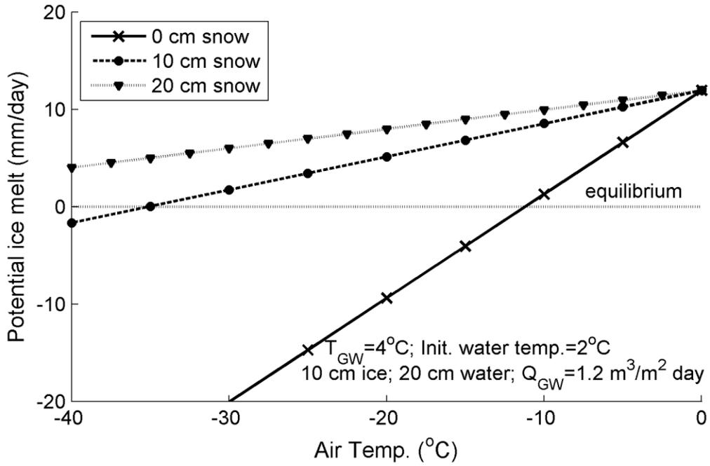
Figure 3.9. Potential ice melt with varying temperatures at different snow depths.
