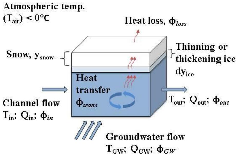
Figure 3.3. Conceptual diagram of groundwater heat affecting river ice thickness in subarctic rivers (see variable definitions in Appendix A3).
