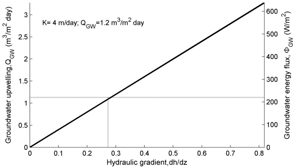
Figure 3.6. Hydraulic gradient relative to the groundwater upwelling rate and its associated heat flux at a groundwater temperature of  $4^\circ\text{C}$  at the measured vertical hydraulic gradient.
