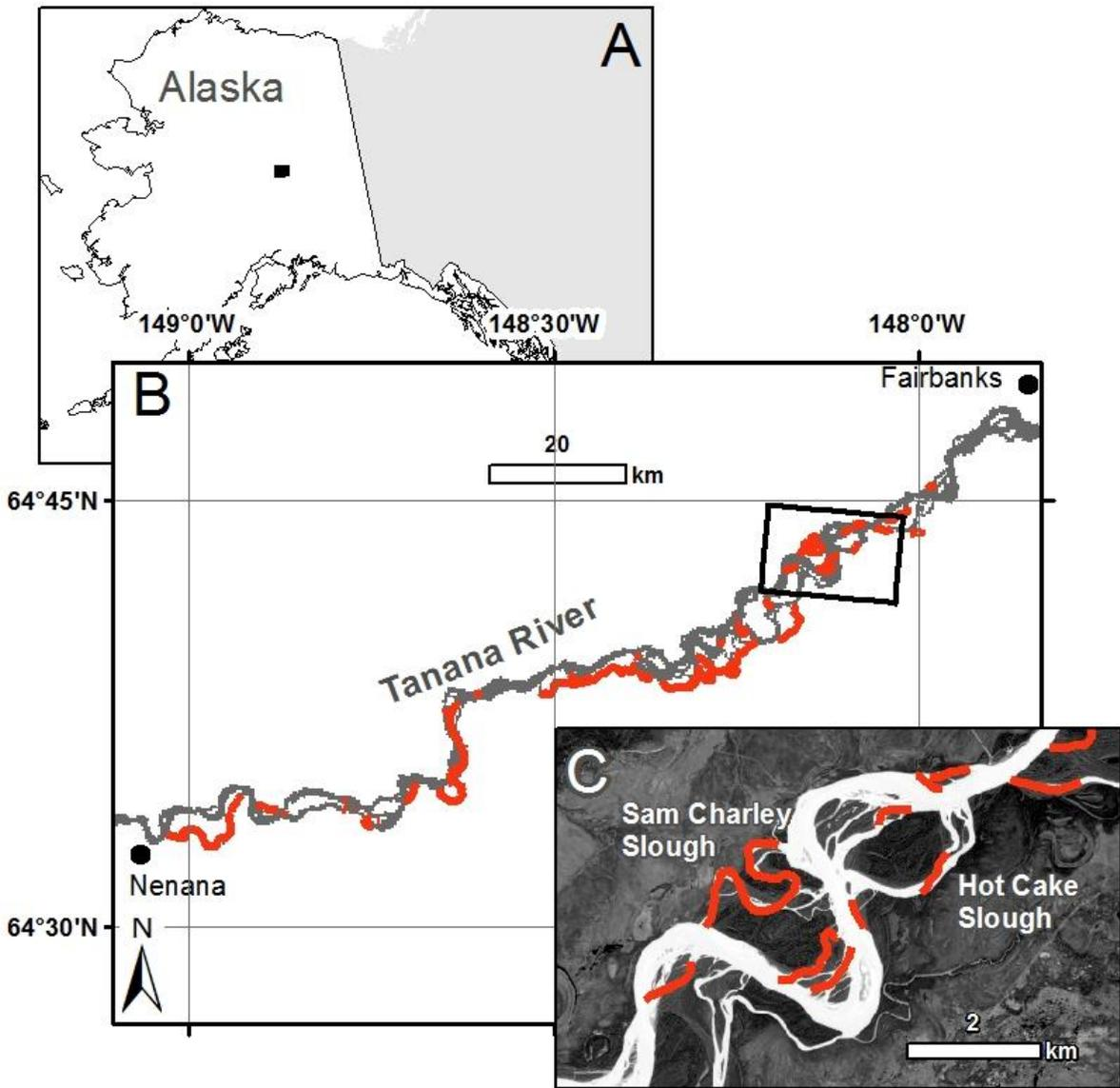
Figure 4.2. Panels A through C identify the location and extent of the study area and the locations of Hot Cake and Sam Charley Sloughs in the Tanana River in Alaska. The areas identified in red were mapped as dangerous according to field surveys. The inset black boxes in panels A and B mark the image extent shown in panels B and C, respectively.
