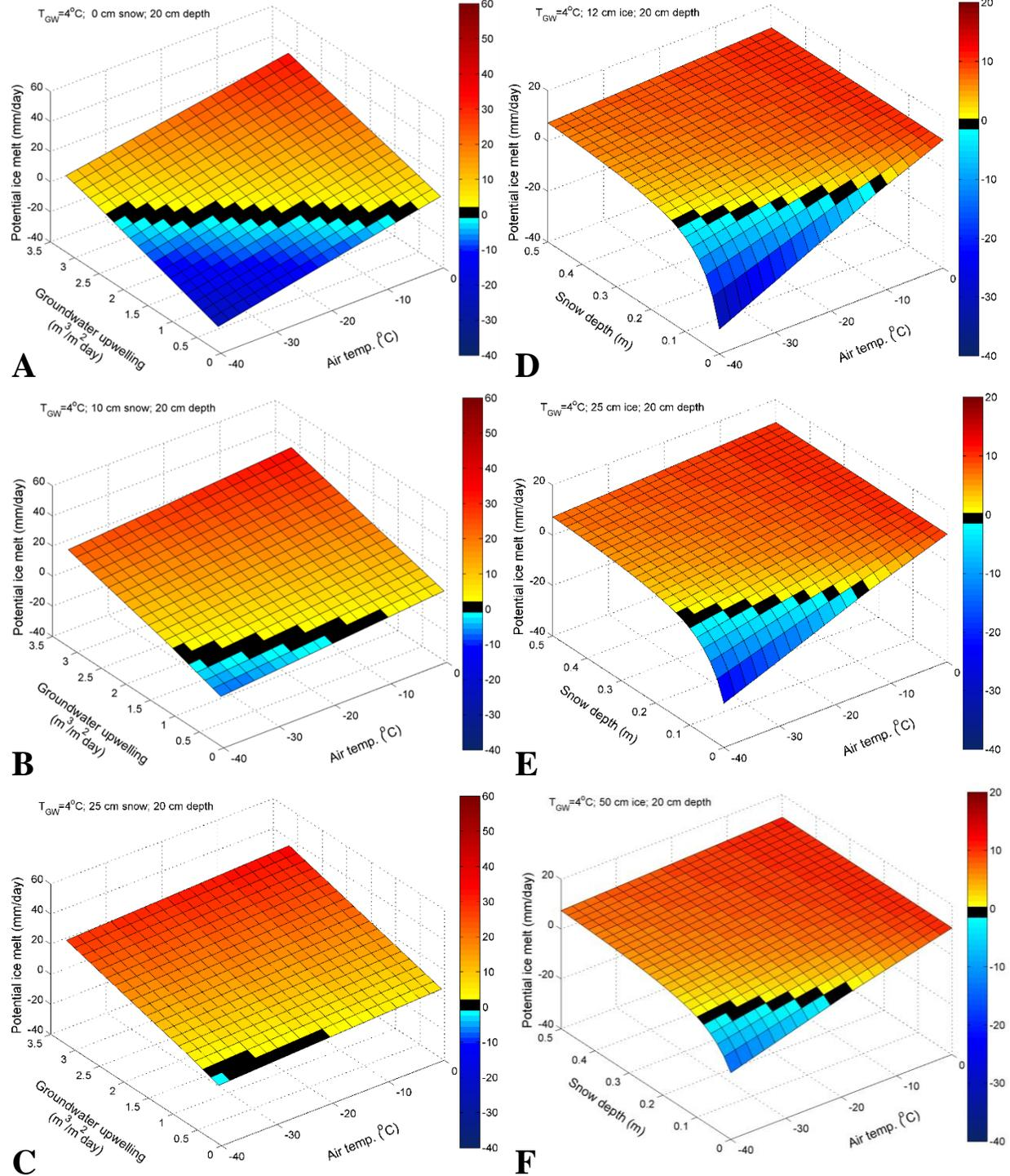
Figure 3.11. A-F. Three dimensional melt rate response curves. Melt rate over a range of air temperatures and groundwater upwelling rates (down the left column) or snow depths (down the right column) given specific initial conditions (noted in the upper left).
