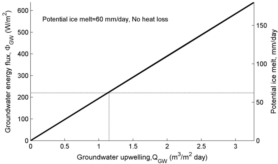
Figure 3.7. Heat flux and potential ice melt associated with variable groundwater upwelling at a temperature of 4°C assuming a system with no atmospheric heat losses or gains (perfectly insulated from the atmospheric temperature).
