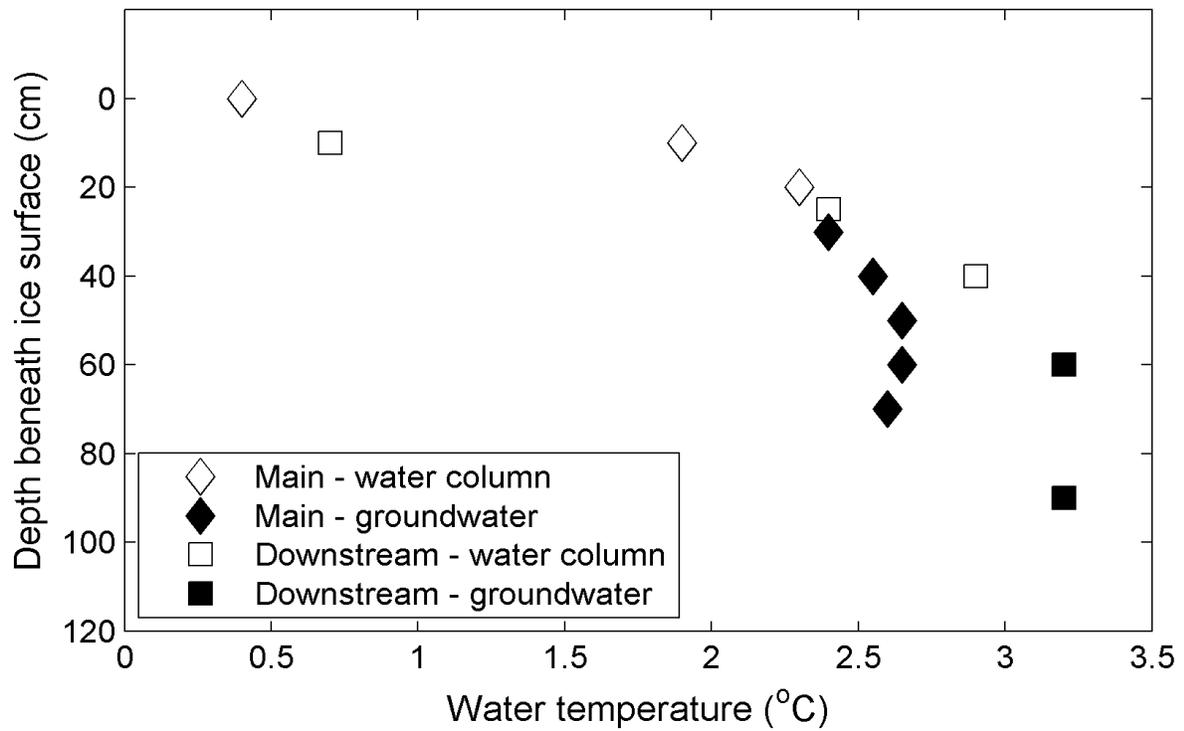
Figure 3.5. Water temperatures in the Hot Cake Slough of the Tanana River (March 19, 2013) at the upstream and downstream monitoring stations.
