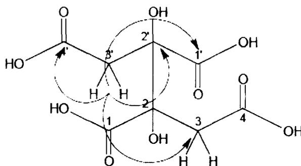
**Figure 16 BBA gHMBC correlations.** The notable correlation between C3 and H3 suggests a long-range coupling due to the symmetry. All four carbons correlate to H3 in gHMBC. Symmetrical correlations are not illustrated for clarity's sake.
