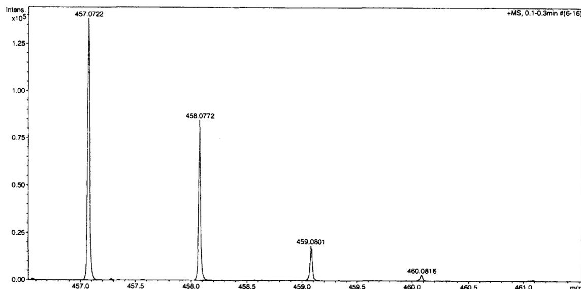
**Figure 14 Positive ion mass spectrometry of DPG.** Results of Q-TOF\_MS with an electrospray ionization source. The main peak at 457.0722  $m/z$  matches the theoretical  $[M-2CO+Na-H+Na]^+$   $m/z$ , and the secondary peak matches the mass predicted from the addition of deuterium from NMR solvent.
