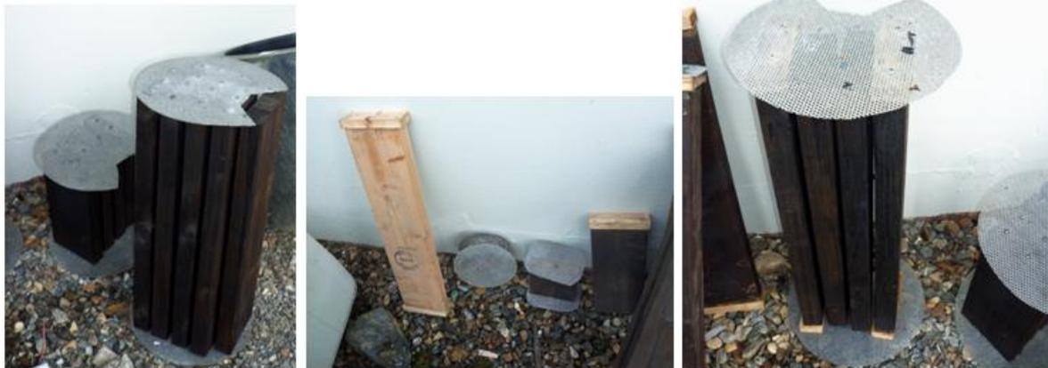
Figure 7: Creosote-treated wood cartridges used in the generator column exposure system.
