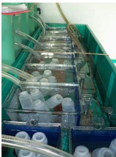
Figure 8: PVC column generator exposure system.
