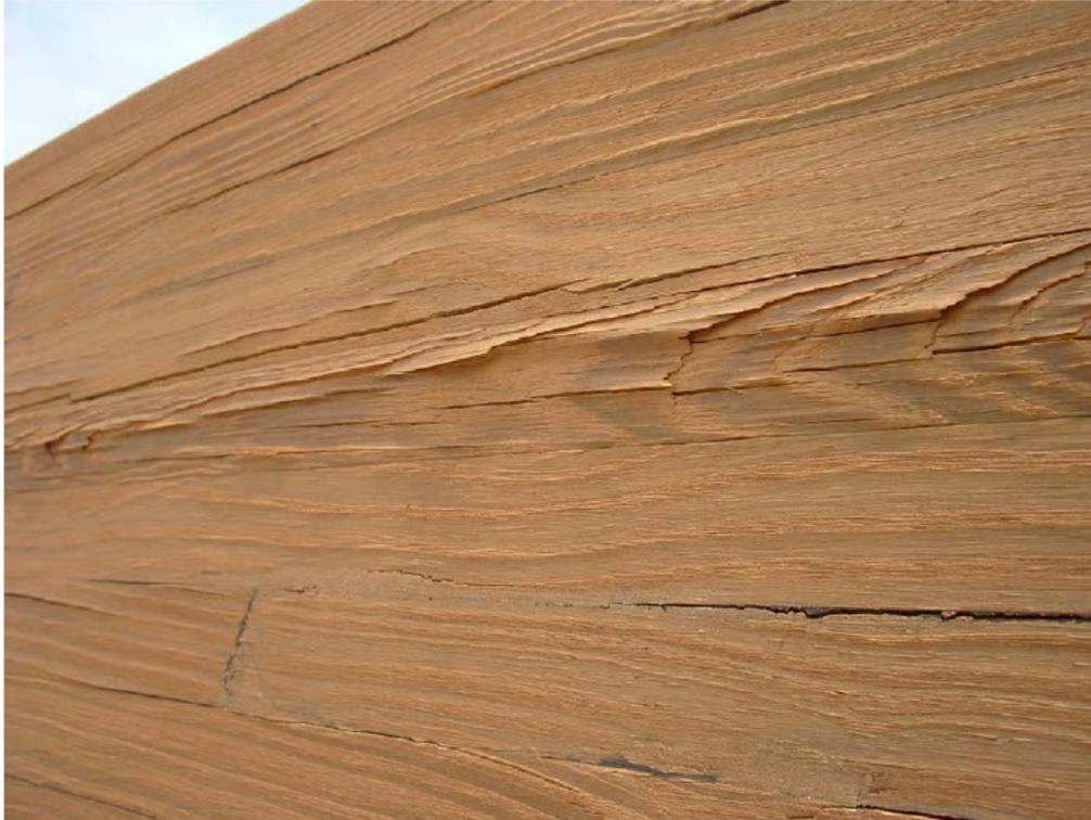
Figure 5.3. Raised grain, shelling, and checking in glulam beam treated with CCA after bonding
