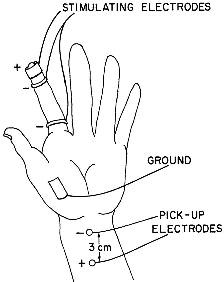
Fig. 6. Wiring diagram used to obtain median nerve conduction velocity measurements from the forefinger
