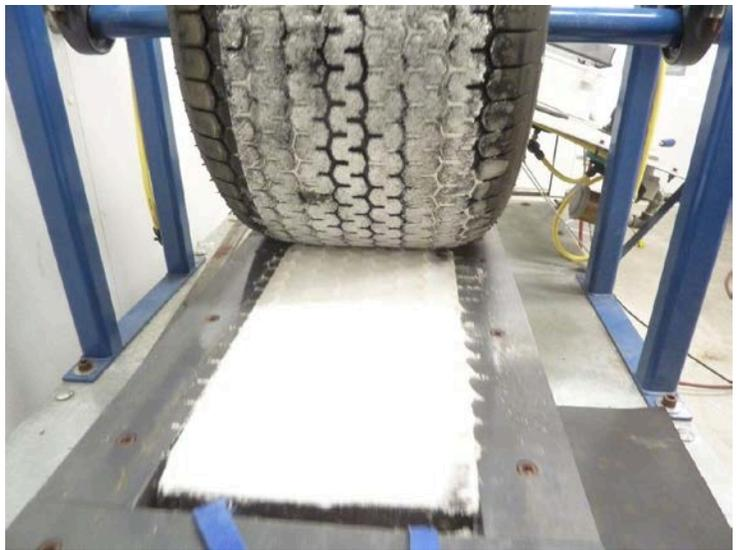
**Figure 1.** Trafficking machine in action in the MSU Subzero Lab.
